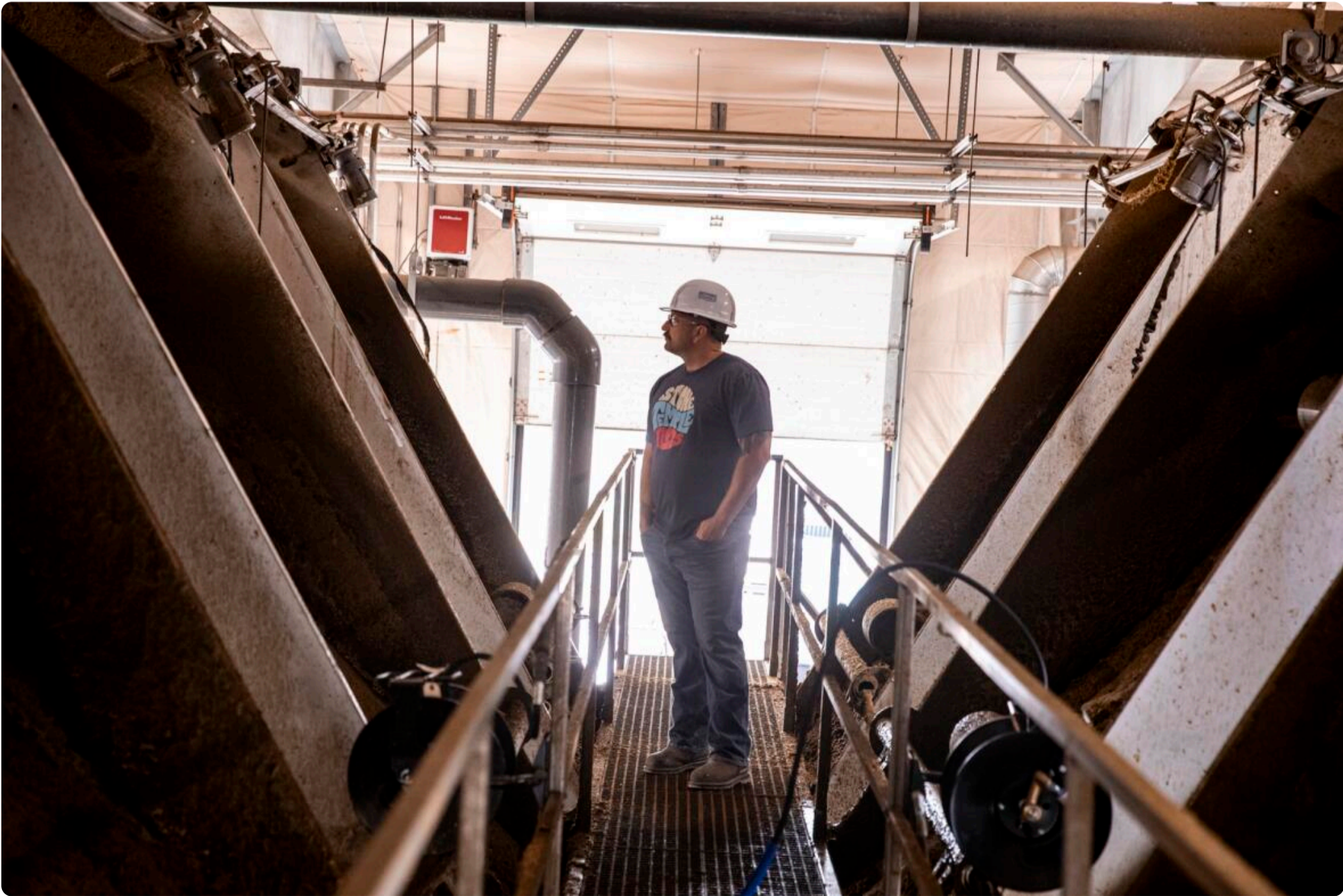
MJ Kelley looks over screen filters at the Marshall Ridge Renewable Energy Center in State Center on Sept. 18. The facility's three anaerobic manure digesters extract methane from dairy cow manure. (Nick Rohlman/The Gazette)
