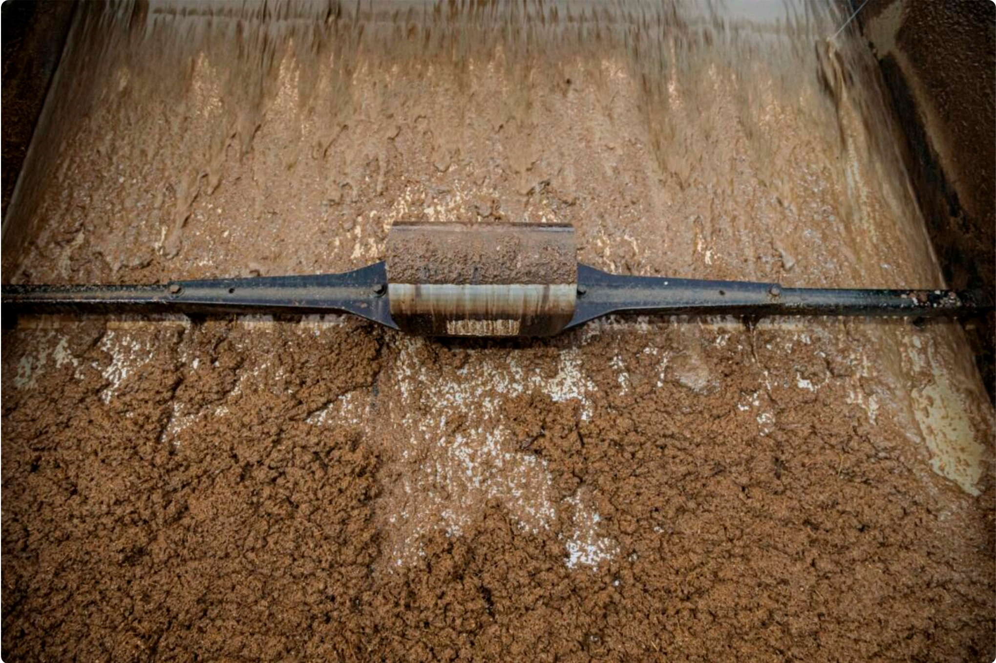
Manure is passed over a screen filter at the Marshall Ridge Renewable Energy Center in State Center on Sept. 18. The facility's three anaerobic manure digesters extract methane from dairy cow manure. (Nick Rohlman/The Gazette)
